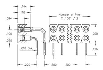
**Description:** Interconnect Socket Right Angle Socket Accepts .015" - .025" (0,38 - 0,635 mm) dia leads Double Row Through Hole Plating Code:
