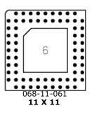
**Description:** PGA Socket Solder Tail PGA Socket Through Hole
