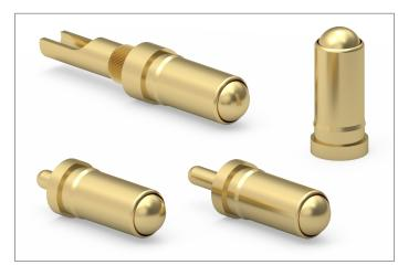
7945-2-15-20-09-14-11-0 has a .118" (3 mm) long tail. The solder-cup version, P/N: 7949-0-15-20-09-14-11-0, is designed to accept wire sizes up to 20 AWG. It has two press-fit features, a barb, and a knurl, allowing the pin to be pressed in from either direction. The knurl, an anti-rotation press-fit feature, is preferred when maintaining solder-cup alignment is critical.
