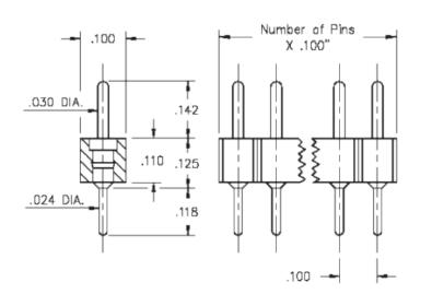
**Description:** Interconnect Header Low Profile Solder Tail Header .030" (0,76mm) Pin Head Single Row Through Hole Plating Code: 10 Shell Plating: 10 µ" Gold over 100 µ" Nickel
