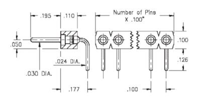
Description: Interconnect Header Right Angle Pin Header .030" (0,76mm) Pin Head Single Row Plating Code: 10
