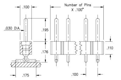
**Description:** Interconnect Header Surface Mount Pin Header .030" (0,76mm) Pin Head Single Row Surface Mount **Plating Code:** 10 Shell Plating: 10 µ" Gold over 100 µ" Nickel
