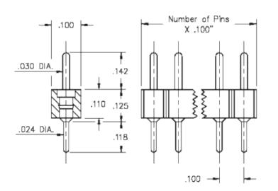
**Description:** Interconnect Header Low Profile Solder Tail Header .030" (0,76mm) Pin Head Single Row Through Hole Plating Code: 10 Shell Plating: 10 µ" Gold over 100 µ" Nickel
