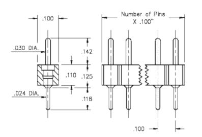
**Description:** Interconnect Header Low Profile Solder Tail Header .030" (0,76mm) Pin Head Single Row Through Hole Plating Code: 10 Shell Plating: 10  $\mu$ " Gold over 100  $\mu$ " Nickel
