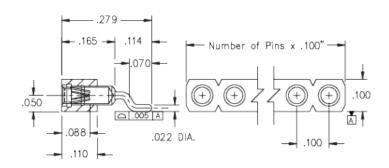
**Description:** Interconnect Socket Horizontal Mount Socket Accepts .025" - .037" (0,635 - 0,94 mm)dia leads Single Row Surface Mount **Plating Code: Shell Plating:** 200 μ" Tin (matte finish) over 100 μ" Nickel
