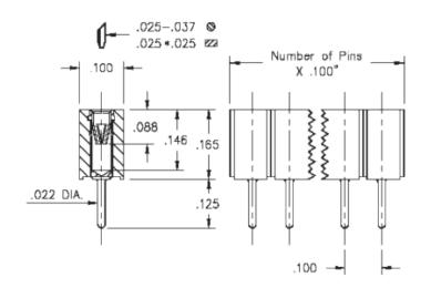
**Description:** Interconnect Socket Standard Solder Tail Socket Accepts .025"- .037" (0,635 - 0,94 mm)dia leads Single Row Through Hole Plating Code: **Shell Plating:**
