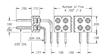
Description: Interconnect Header Right Angle Pin Header .030" (0,76mm) Pin Head Double Row Through Hole Plating Code: 10 Shell Plating: 10 μ" Gold over 100 μ" Nickel
