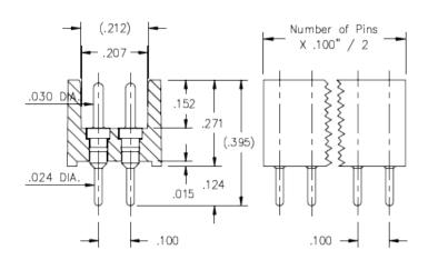
**Description:** Interconnect Header Shrouded Pin Header .030" (0,76mm) Pin Head Double Row Through Hole Plating Code: 10 Shell Plating: 10  $\mu$ " Gold over 100  $\mu$ " Nickel
