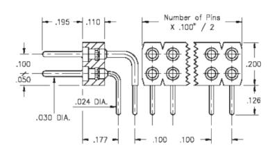
**Description:** Interconnect Header Right Angle Pin Header .030" (0,76mm) Pin Head Double Row Through Hole Plating Code: 10 Shell Plating: 10 µ" Gold over 100 µ" Nickel
