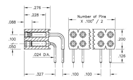
**Description:** Interconnect Socket Right Angle Socket Accepts .025" - .037" (0,635 - 0,94 mm)dia leads Double Row
