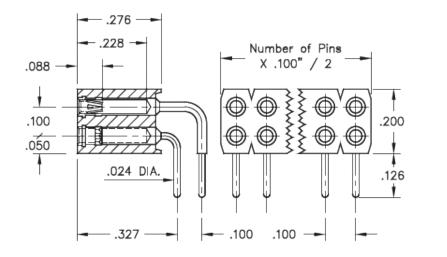
Interconnect Socket Right Angle Socket Accepts .025"- .037" (0,635 - 0,94 mm)dia leads Double Row Through Hole Plating Code: 43 Shell Plating: 200 µ" Tin (matte finish) over 100 µ" Nickel Inner Contact Plating:
