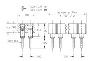
**Description:** Interconnect Socket Standard Solder Tail Socket Accepts .025"- .037" (0,635 - 0,94 mm)dia leads Double Row Through Hole Plating Code: 43 Shell Plating: 200 µ" Tin (matte finish) over 100 µ" Nickel Inner Contact Plating:
