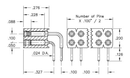
**Description:** Interconnect Socket Right Angle Socket Accepts .025" - .037" (0,635 - 0,94 mm)dia leads Double Row Through Hole
