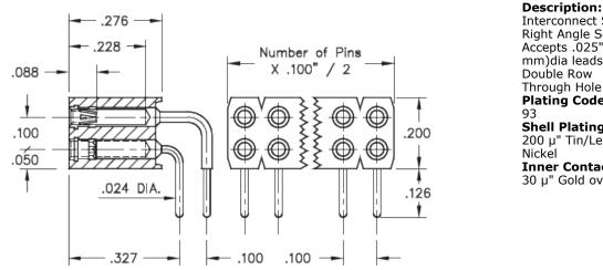
Interconnect Socket Right Angle Socket Accepts .025"- .037" (0,635 - 0,94 mm)dia leads Double Row Through Hole Plating Code: Shell Plating: 200 μ" Tin/Lead(93/7) over 100 μ" Nickel Inner Contact Plating:
