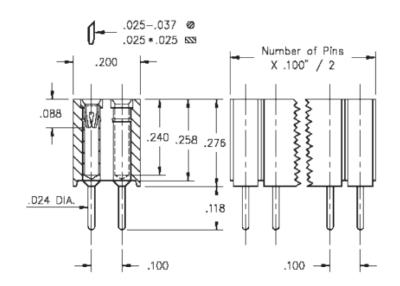
**Description:** Interconnect Socket Standard Solder Tail Socket Accepts .025" - .037" (0,635 - 0,94 mm)dia leads
