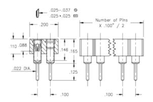
Description: Interconnect Socket Standard Solder Tail Socket Accepts .025"- .037" (0,635 - 0,94 mm)dia leads Double Row Through Hole Plating Code: 93 Shell Plating: 200 μ" Tin/Lead(93/7) over 100 μ" Nickel Inner Contact Plating:
