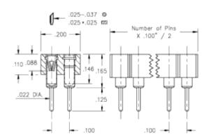
Description: Interconnect Socket Standard Solder Tail Socket Accepts .025"- .037" (0,635 - 0,94 mm)dia leads Double Row Through Hole Plating Code: 93 Shell Plating: 200 μ" Tin/Lead(93/7) over 100 μ" Nickel Inner Contact Plating: 30 µ" Gold over 50 µ" Nickel
