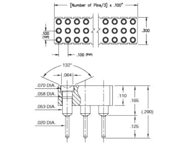
**Description:** Interconnect Concave Face Target Connector Spring-Loaded Header Vertical Mount Through Hole Target with Concave Face Triple Row Through Hole Plating Code: 10 Shell Plating: 10 µ" Gold over 100 µ" Nickel Packaging: Packaged in Bulk
