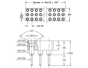
**Description:** Interconnect Target Connector Spring-Loaded Header Vertical Mount Through Hole Target with Concave Face Triple Row Through Hole Plating Code: 10 Shell Plating: 10 µ" Gold over 100 µ" Nickel
