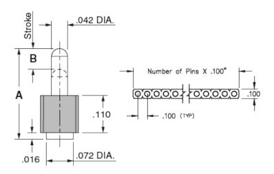
**Description:** Interconnect SLC Header Spring-Loaded Header Vertical Mount SMT Single Row Surface Mount **Plating Code:** Shell Plating: 20μ" Gold over 100μ" Nickel
