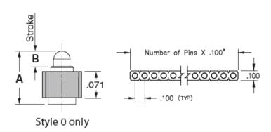
**Description:** Interconnect SLC Header Spring-Loaded Header Vertical Mount SMT Single Row Surface Mount **Plating Code:** Shell Plating:  $20\mu$ " Gold over  $100\mu$ " Nickel Inner Spring Plating: 10µ" Gold
