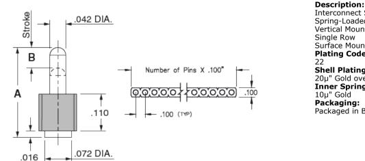
Interconnect SLC Header Spring-Loaded Header Vertical Mount SMT Single Row Surface Mount **Plating Code:** 22 **Shell Plating:** 20µ" Gold over 100µ" Nickel **Inner Spring Plating:** 10µ" Gold **Packaging:** Packaged in Bulk
