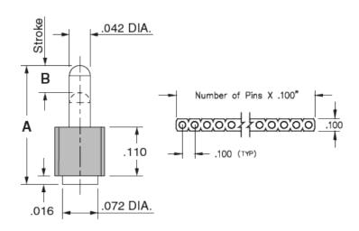
**Description:** Interconnect SLC Header Spring-Loaded Header Vertical Mount SMT Single Row Surface Mount **Plating Code:**
