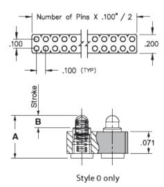
**Description:** Interconnect SLC Header Spring-Loaded Header Vertical Mount SMT Double Row Surface Mount **Plating Code:** Shell Plating:  $20\mu$ " Gold over  $100\mu$ " Nickel Inner Spring Plating: 10μ" Gold Packaging:
