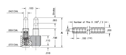
**Description:** Interconnect SLC Header Spring-Loaded Header Vertical Mount SMT Double Row Surface Mount Plating Code: 22 Shell Plating: 20µ" Gold over 100µ" Nickel Inner Spring Plating: 10µ" Gold Packaging: Packaged in Bulk
