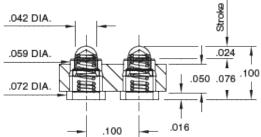
Description: Interconnect SLC Header Spring-Loaded Header Vertical Mount SMT Double Row Surface Mount Plating Code: 22 Shell Plating: 20µ" Gold over 100µ" Nickel Inner Spring Plating: 10µ" Gold Packaging: Packaged in Bulk
