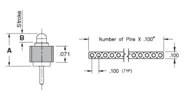
**Description:** Interconnect SLC Header Spring-Loaded Header Vertical Mount Through-Hole Single Row Through Hole Plating Code: 22 Shell Plating: 20µ" Gold over 100µ" Nickel Inner Spring Plating: 10µ" Gold
