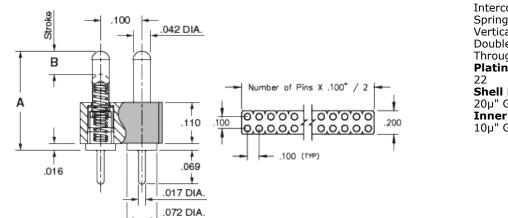
Description: Interconnect SLC Header Spring-Loaded Header Vertical Mount Through-Hole Double Row Through Hole Plating Code: 22 Shell Plating: 20µ" Gold over 100µ" Nickel Inner Spring Plating: 10µ" Gold
