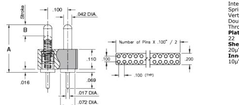
**Description:** Interconnect SLC Header Spring-Loaded Header Vertical Mount Through-Hole Double Row Through Hole Plating Code: Shell Plating: 20µ" Gold over 100µ" Nickel Inner Spring Plating: 10µ" Gold
