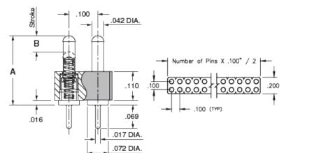
**Description:** Interconnect SLC Header Spring-Loaded Header Vertical Mount Through-Hole Double Row Through Hole Plating Code: 22 Shell Plating: 20µ" Gold over 100µ" Nickel Inner Spring Plating: 10µ" Gold
