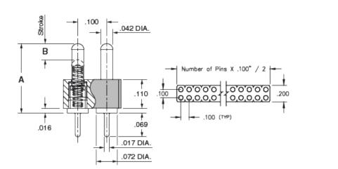
**Description:** Interconnect SLC Header Spring-Loaded Header Vertical Mount Through-Hole Double Row Through Hole Plating Code: 22 Shell Plating: 20µ" Gold over 100µ" Nickel Inner Spring Plating: 10µ" Gold
