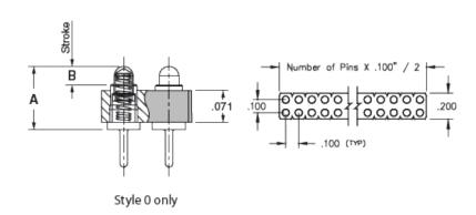
**Description:** Interconnect SLC Header Spring-Loaded Header Vertical Mount Through-Hole Double Row Through Hole Plating Code:
