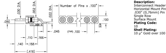
Horizontal Mount Pin Header .030" (0,76mm) Pin Head 10  $\mu$ " Gold over 100  $\mu$ " Nickel
