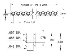
**Description:** Interconnect Target Connector Spring-Loaded Header Vertical Mount SMT Target Single Row Surface Mount Plating Code: 10 Shell Plating: 10 µ" Gold over 100 µ" Nickel Packaging: Packaged in Bulk
