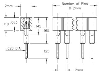
Interconnect Socket Standard Solder Tail Socket Accepts .015"- .026" (0,38 - 0,66 mm) dia leads Single Row Through Hole Plating Code: 43 Shell Plating: 200 µ" Tin (matte finish) over 100 µ" Nickel Inner Contact Plating: 30 µ" Gold over 50 µ" Nickel
