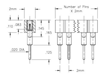
**Description:** Interconnect Socket Standard Solder Tail Socket Accepts .015"- .026" (0,38 - 0,66 mm) dia leads Single Row Through Hole Plating Code: 93 Shell Plating: 200 μ" Tin/Lead(93/7) over 100 μ" Nickel Inner Contact Plating: 30 µ" Gold over 50 µ" Nickel
