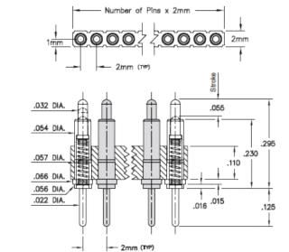
**Description:** Interconnect SLC Header Spring-Loaded Header Vertical Mount Through-Hole Single Row Through Hole Plating Code: 22 Shell Plating: 20µ" Gold over 100µ" Nickel Inner Spring Plating: 10µ" Gold Packaging: Packaged in Bulk
