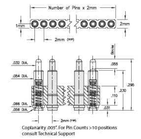
Description: Interconnect SLC Header Spring-Loaded Header Vertical Mount SMT Single Row Surface Mount Plating Code: 22 Shell Plating: 20µ" Gold over 100µ" Nickel Inner Spring Plating: 10µ" Gold Packaging: Packaged in Bulk
