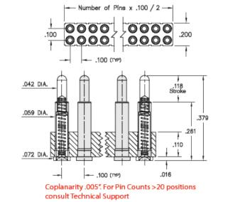
**Description:** Interconnect SLC Header Spring-Loaded Header Vertical Mount SMT Double Row Surface Mount Plating Code: 22 Shell Plating: 20µ" Gold over 100µ" Nickel Inner Spring Plating: 10µ" Gold Packaging: Packaged in Bulk
