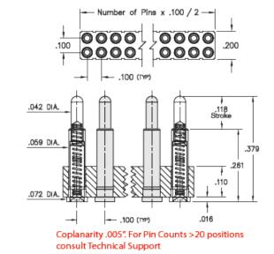
Description: Interconnect SLC Header Spring-Loaded Header Vertical Mount SMT Double Row Surface Mount Plating Code: 22 Shell Plating: 20µ" Gold over 100µ" Nickel Inner Spring Plating: 10µ" Gold Packaging: Packaged in Bulk
