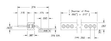
Coplanarity .005". For Pin Counts >20 positions consult Technical Support. Description: Interconnect Header Surface Mount Pin Header .016" (0,41mm) Pin Head Single Row Surface Mount Plating Code: 10 Shell Plating: 10 μ" Gold over 100 μ" Nickel
