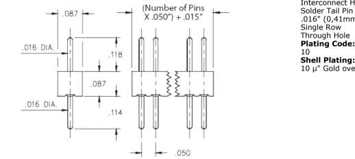
**Description:** Interconnect Header Solder Tail Pin Header .016" (0,41mm) Pin Head Plating Code: Shell Plating: 10  $\mu$ " Gold over 100  $\mu$ " Nickel
