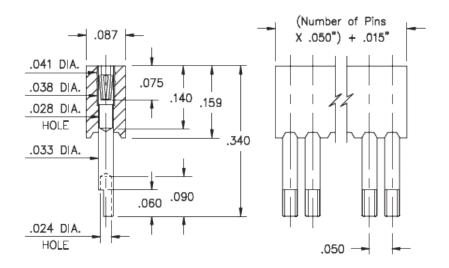
**Description:** Interconnect Socket Solder Cup Strip Socket Accepts .015"- .020" (0,38 - 0,508 mm) dia leads Single Row Through Hole
