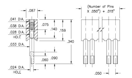
**Description:** Interconnect Socket Solder Cup Strip Socket Accepts .015"- .020" (0,38 - 0,508 mm) dia leads Single Row Through Hole Plating Code:
