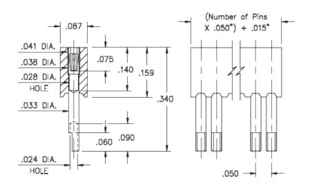
**Description:** Interconnect Socket Solder Cup Strip Socket Accepts .015"- .020" (0,38 - 0,508 mm) dia leads Single Row Through Hole Plating Code: Shell Plating:
