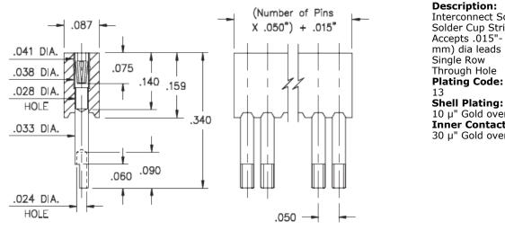
Interconnect Socket Solder Cup Strip Socket Accepts .015"- .020" (0,38 - 0,508 mm) dia leads Through Hole Plating Code:
